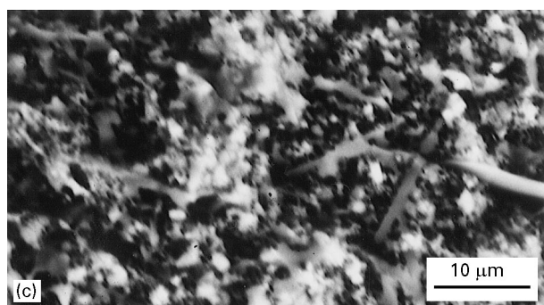
Figure 5 (a)–(d) SEM fractographs showing grain growth as a function of temperature for the samples with 2.0 wt % B addition. (a) 1900 °C; (b) 2050 °C; (c) 2100 °C (densified to 80.5%); (d) 2170 °C.
